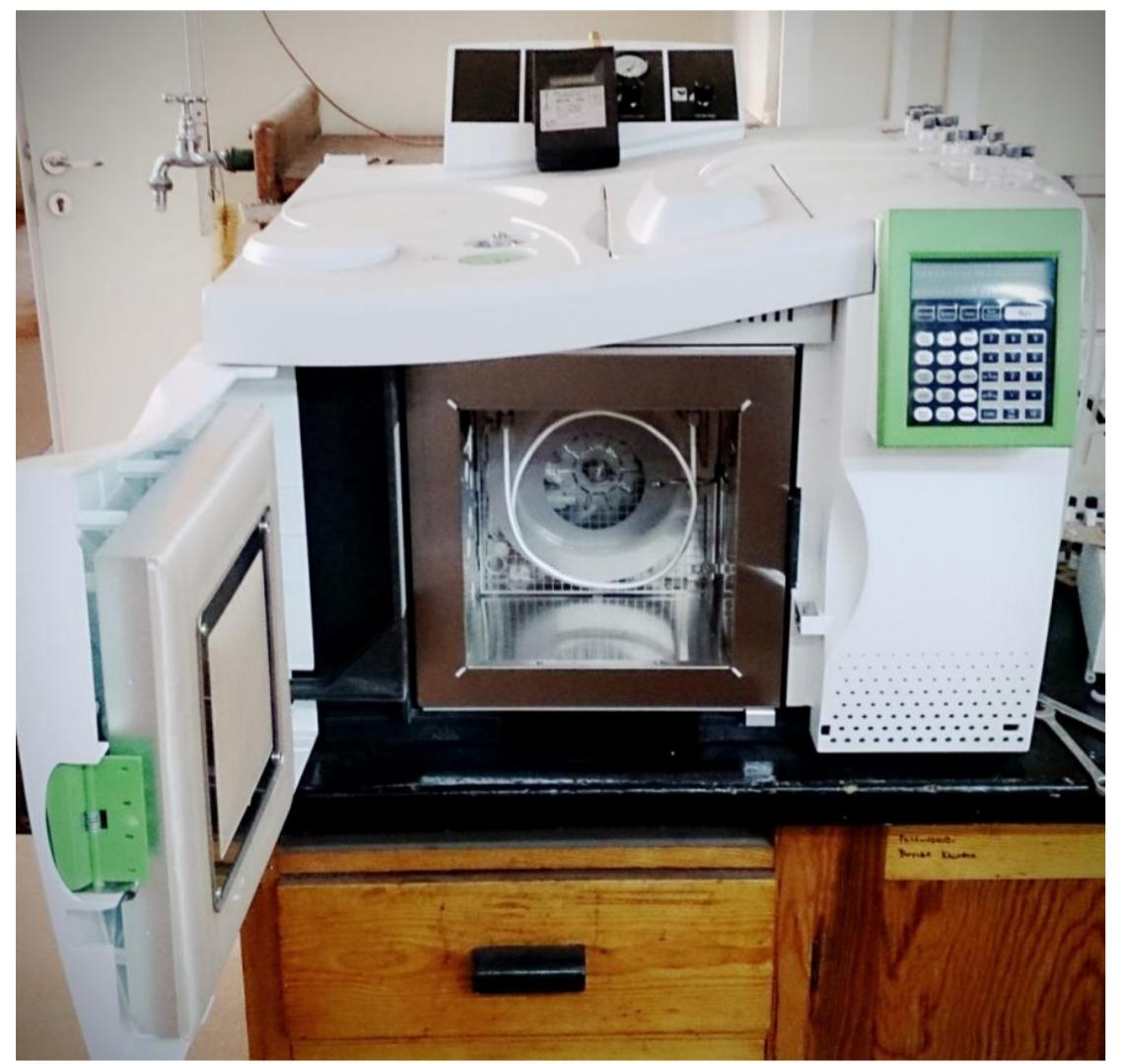
Pic. 1 Gas chromatograph with TCD detector Clarus 480, Perkin Elmer corp.
