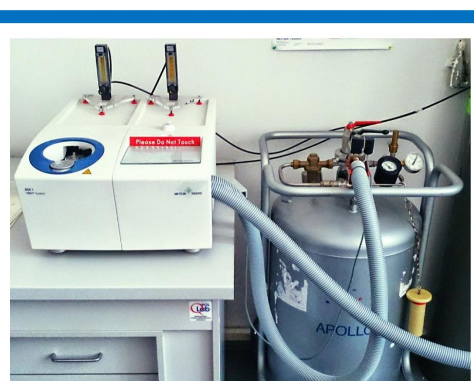
Pic. 2 Differential scanning calorimeter DSC 1, Mettler Toledo corp.
